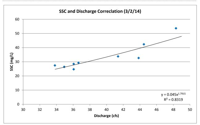
The SSC and discharge correlation shown in Figure 20 was used to generate estimated SSC values during the time period that was not monitored from 10:00 on March 2 to 00:00 on March 3. The measured SSC values are from the last portion of the hydrograph. See Figure 17. The equation: **SSCpredicted** =  $0.045X^{1.7915}$  where X is discharge, was used to calculate predicted SSC values for the time period above.
