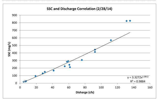
The SSC and discharge correlation shown in Figure 19 was used to generate estimated SSC values during the time period that was not monitored from 11:00 to 22:30 on February 28. The measured SSC values are from the center portion of the hydrograph. See Figure 17. The equation: **SSCpredicted** =  $3.3272X^{1.0812}$  where X is discharge, was used to calculate predicted SSC values for the time period above.
