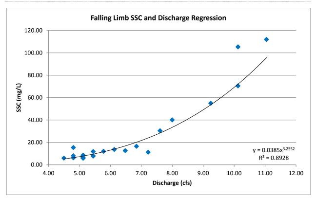
The SSC and discharge correlation (shown in Figure 13) was utilized to generate estimated SSC values during the time period that was not monitored from 10:30 on March 2 to 00:00 on March 3. The measured SSC values were from the falling limb of the hydrograph. See Figure 11. The equation: **SSCpredicted** =  $0.0385X^{3.2552}$  where X is discharge, was used to calculate predicted SSC values.
