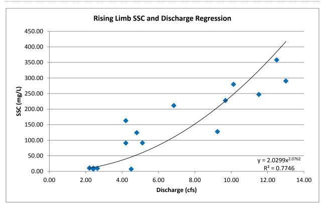
The SSC and discharge correlation (shown in Figure 12) was used to generate estimated SSC values during the time period that was not monitored from 16:00 on February 26 to 22:00 on February 27. The measured SSC values were from the rising limb of the hydrograph. See Figure 11. The equation: **SSCpredicted** = **2**.**0299X**<sup>2.0762</sup> where X is discharge, was used to calculate predicted SSC values for the time period referenced above.
