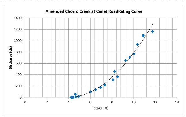
Figure 7 shows the amended rating curve with the removal of three data points and the addition of 15 low flow discharge values. Discharge for stage heights below 12.10 feet can be approximated by: **Q** (cfs) = 20.907Y<sup>2</sup> - 5.8341Y where Y is the depth of water (in feet, recorded by the bubbler gauge) minus channel bottom elevation (3.75 ft) above the reference datum. This equation was used in the sediment load analysis of this report.
