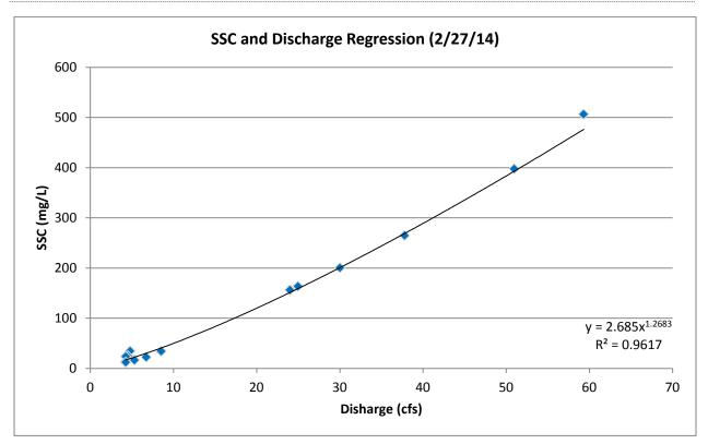
The SSC and discharge correlation (shown in Figure 18) was used to generate estimated SSC values during the time period that was not monitored from 5:00 to 21:30 on February 27. The measured SSC values are from the first portion of the hydrograph. See Figure 17. The equation: **SSCpredicted** = 2.685X<sup>1.2683</sup> where X is discharge, was used to calculate predicted SSC values for the time period above.
