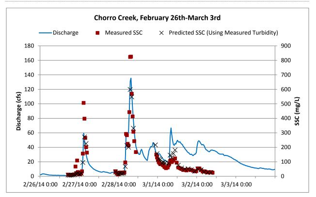
FIGURE 25: CHORRO CREEK MEASURED SSC AND PREDICTED SSC USING TURBIDITY
