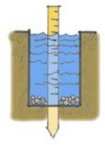
4. Pour water into the holes at least  $8^{\circ}$ -10° above the gravel. Using a stake marked at  $\frac{1}{4}^{\circ}$  intervals, measure water level drop at 30 minute intervals. Refill after each measurement.
