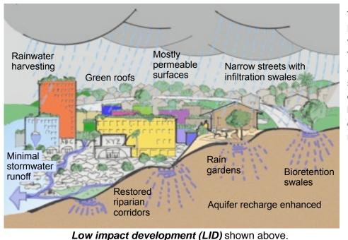
The basic LID strategy for handling runoff is to reduce the volume and decentralize flows. This is usually best accomplished by creating a series of smaller retention and detention areas that allow localized infiltration instead of carrying stormwater runoff to remote collection areas to be treated. This is accomplished by specific LID techniques, shown in recipe cards A-H, to perform the LID functions listed above.
