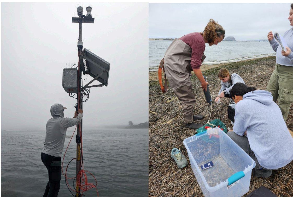
Figure 24. Senior research scientist Ian Robbins checks on the instruments at the back bay sensor station (left). The top of the station houses meteorological instruments for measuring weather parameters and a solar panel to power all the sensors. Dr. Bockmon and her students collect water from Pasadena Park using a Niskin sampler (right). Photos courtesy of Ian Robbins and Dr. Emily Bockmon.
