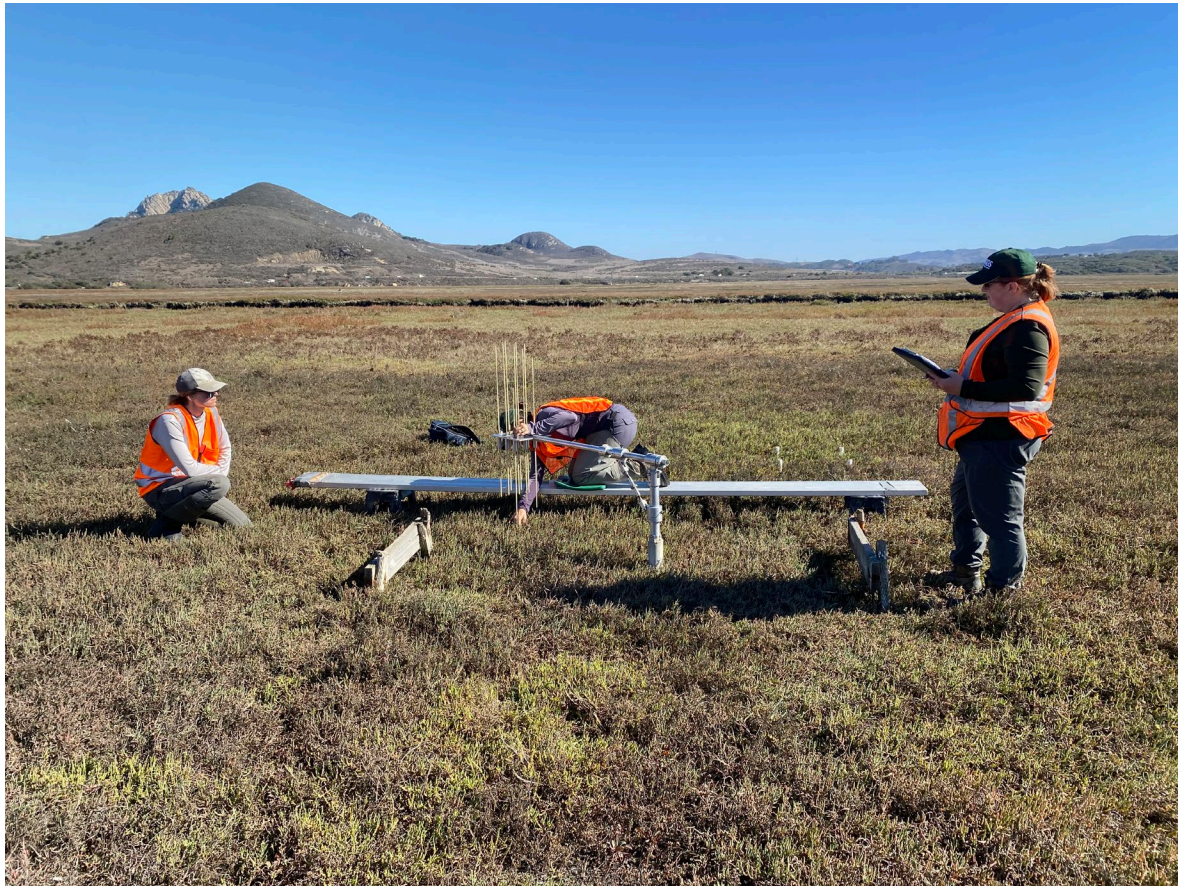
Figure 2. Surface elevation table monitoring near Chorro Creek by USGS. Photo credit: Carolyn Geraghty
