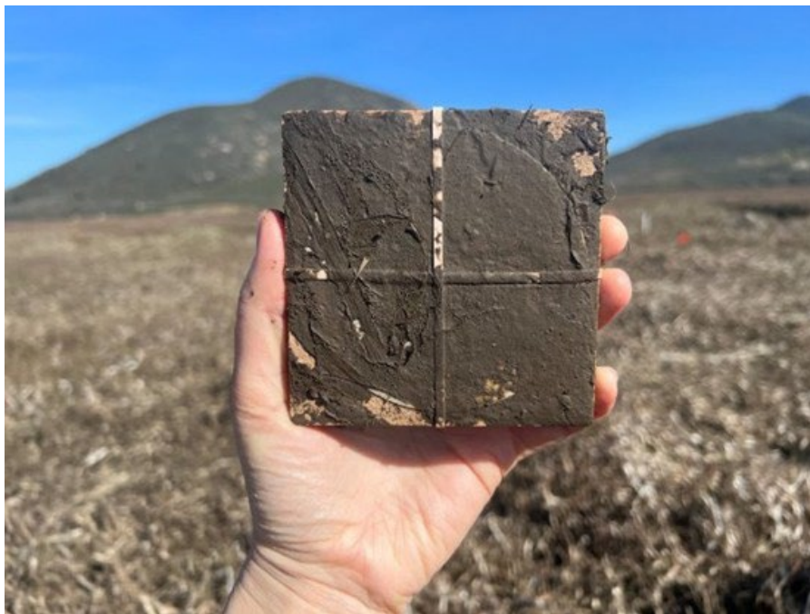
Figure 7. Sediment deposition pad placed in marsh to track seasonal deposition patterns. Photo credit: Jenn Fields.
